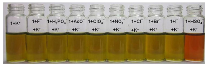
Fig. 4. Color changes induced by the addition of \text{K}^+ (75 equiv.) to a \mathbf{1} \cdot \text{anion} (75 equiv.) complex. [\mathbf{1}] = 4 \times 10^{-4} \text{ M} .
